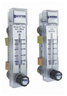
Bass Instruments, PMBC Series Miniature Acrylic Flow meters are low cost and small size flow meters designed to measure instant flow of gases such as air and nitrogen. With the standard adjustment valve, you can fix the flow to the desired amount. Connection parts can be made of optional AISI 316 material.
